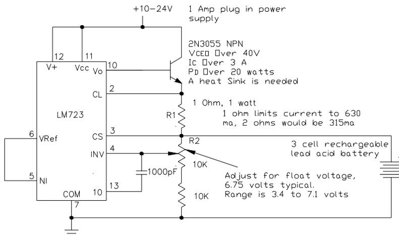
This circuit will begin bulk charging at 630ma the current limit setting until the battery voltage approaches the float voltage. As the float voltage approaches the current is reduced and when the battery voltage equals the float voltage charging stops.
